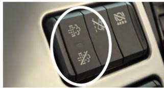
Note: Remember to reset the DPF switch once back under normal conditions and worth checking this is in the normal running position as part of your vehicle checks
