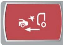
AEBS uses a radar sensor, mounted behind the front grille - to recognise stationary vehicles, or slower moving vehicles which are travelling in the same direction as your unit.
