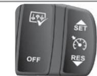
To adjust the speed setting **press once for 1kph or hold for 5kph increments,** and to cancel Cruise Control, press "OFF".
