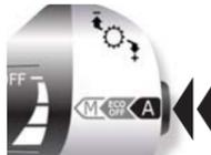
It is possible to temporarily disable EcoMode by **pressing the button on the end of the right hand stalk.** By pressing once, the acceleration and shifting strategy changes to allow the engine to operate at a higher rpm increasing vehicle performance. **Ecomode is then disabled for a minimum of 60 seconds** (or until no longer required) which also allows manual shifting of the gearbox.
