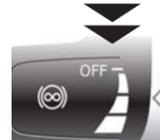
The power of the MX engine brake can be **further enhanced** by downshifting gears to keep the engine speed in the **blue-band of the rev counter.**
