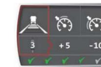
**DSC:** Can be set between **15 and 3.** 15 being the maximum speed allowed above the Cruise Set Speed. The higher this setting the more EcoRoll will engage - **but be aware of speed limits!**
