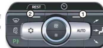
When REST appears in the screen and with the engine off you can select using switch 2 **to give up to 45 minutes** of heat from the engine.
