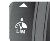
To engage this feature simply **press** at the required speed and you will not be able to exceed the speed **during normal driving.**
